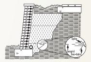
When placing the PVC insert into the back slot you will obtain an inclined wall.
