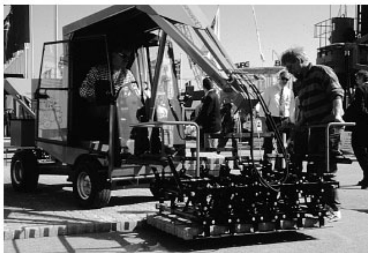
Figure 4. (right) Motorized equipment with a mechanical clamp.
