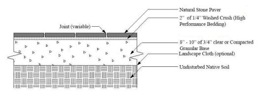
Once the area has been dug down to undisturbed native soil the optional landscape cloth can be installed, followed by the compacted granular base material (refer to image above). This material is then compacted well to provide a strong base.
