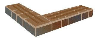
Place the split unit on a well compacted and levelled foundation with the chiselled face expose. Continue the installation as illustrated below. Having previously prepared opposite-angled units, you can now complete the second course using regular blocks.
