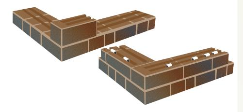
When building higher walls involving a 90° corner, the first geogrid should be installed on one course, followed by the next geogrid, going in the other direction, on the next course. Always keep at least 3 inches of aggregate between the layers of grid. For more information, or details regarding your specific project, please feel free to contact us.
